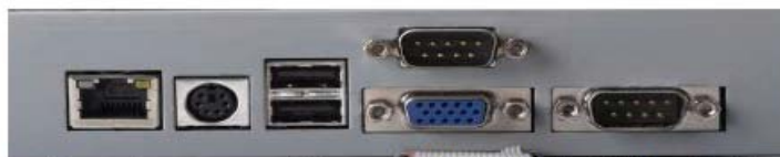
Screw type power Ethernet PS2 USB VGA Serial
