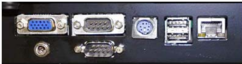
VGA out DC power jack 2-Serial PS2 2-USB Gigabit Ethernet
